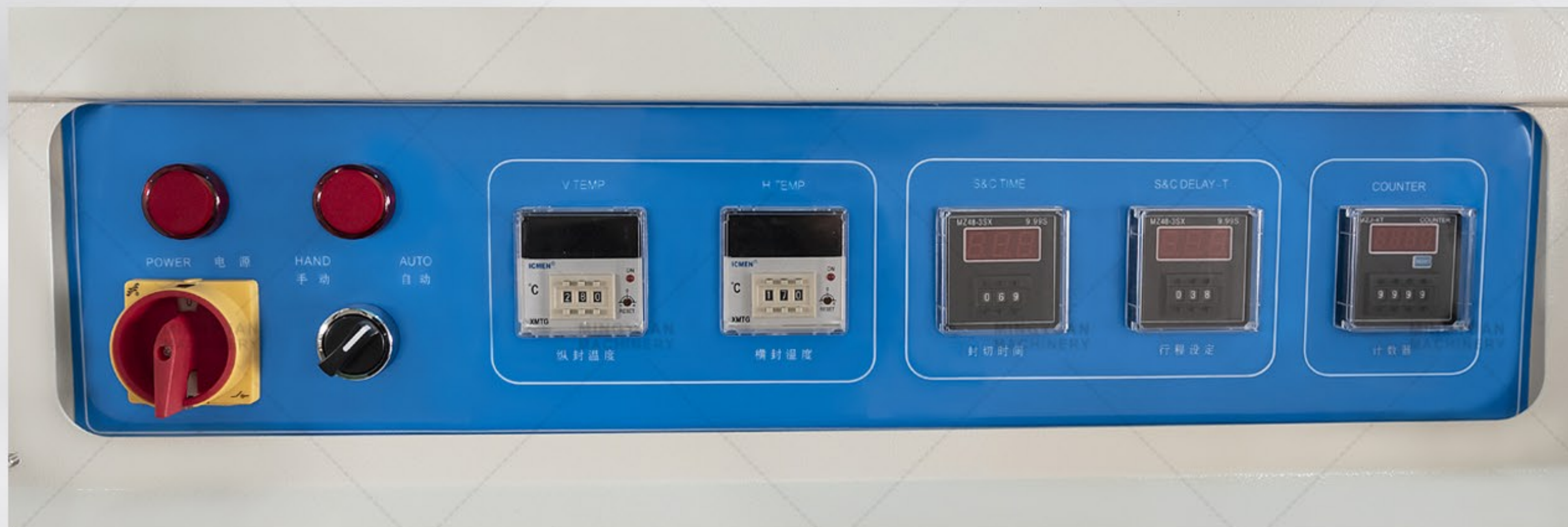
Automatic Heat Shrink Tunnel Wrapping Machine Control Panel
